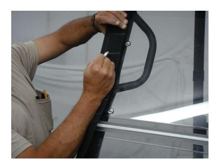
**Step 7:** Cut the webbing strip with household scissors. **AGAIN, DO NOT CUT INTO THE BINDING.** Seal the frayed edges with a lighter. Have a wet cloth handy to dab the edges if needed.
