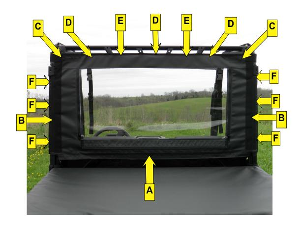
**Step 6:** The webbing/Velcro strip that runs the length of the front roll bars will need to be cut to accommodate the windshield clamps and the grab handle. With chalk, mark the webbing strip where cuts will be made. **DO NOT CUT INTO THE BINDING.**
