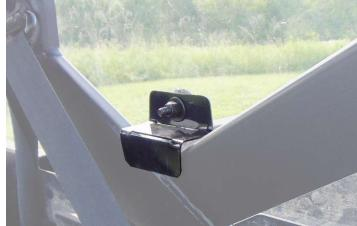
**Step 5:** OPTIONAL-Additional hardware is provided to use in the remaining holes that correspond to holes in the frame. However, some of the bolt holes are difficult to access from the inside of the cab. Install the additional bolts only if more support is desired.
