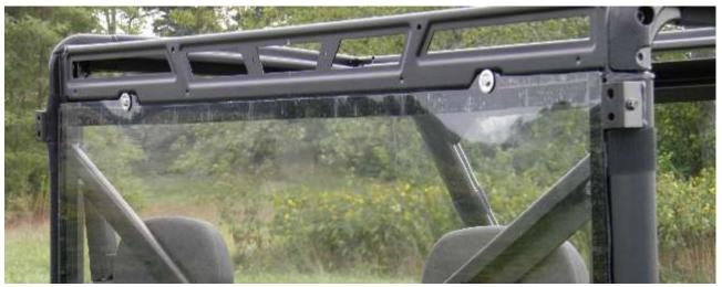
**Step 6:** After all clamps and hardware are attached, tighten the lock nuts on each bolt.
