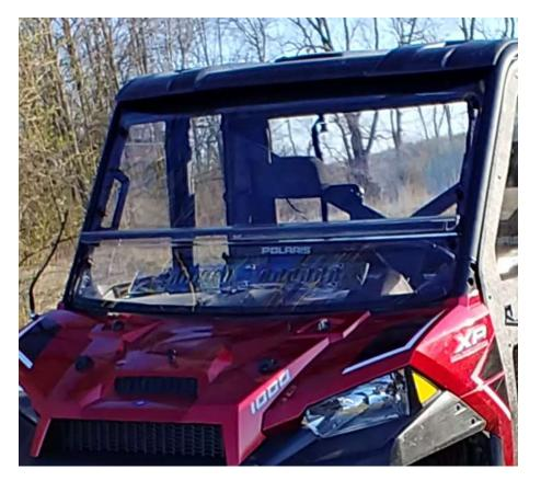
**Step 8:** When satisfied that the upper windshield section is positioned properly, tighten the knob bolts. Attach nuts to the knob bolts to hold in place.
