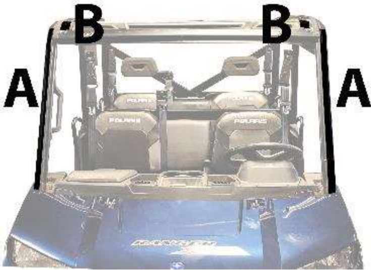
Figure 1: Place adhesive Velcro as shown in photo. This photo shows the placement of the 2" Velcro for Strips A.
