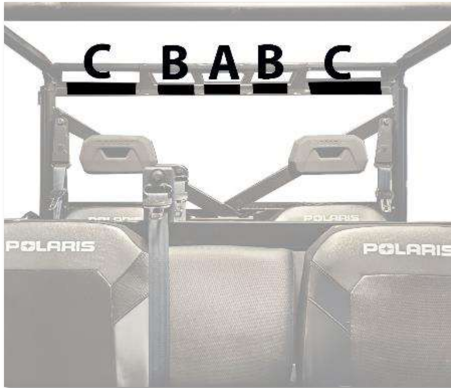
Figure 1: Align the top of the back panel up in the center of the roll bar. Wrap tabs through the openings in the top of the roll cage.
