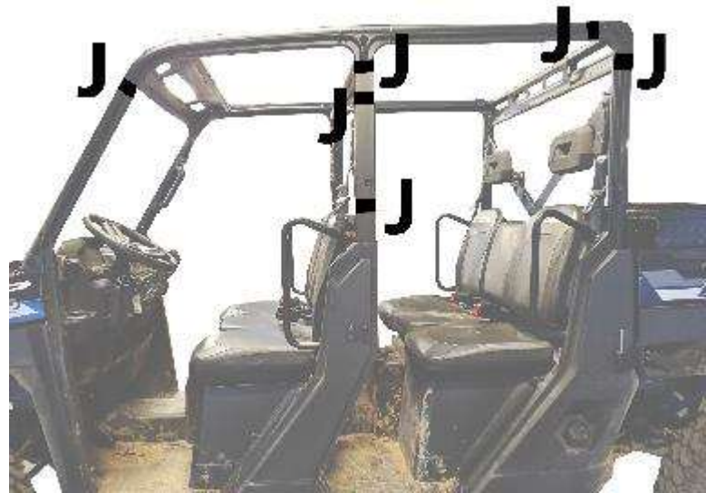
Figure 4: Wrap each adhesive strip J around the roll bar.
