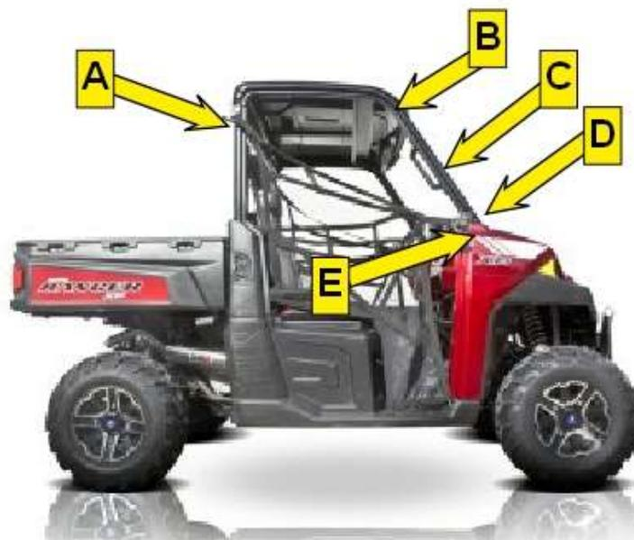
**Step 3:** After all adhesive hook strips are attached, begin attaching the enclosure to the cab frame. As you attach the hook and loop, square each panel to the frame. **PLEASE NOTE, FOR MAXIMUM ADHESION, ALLOW THE ADHESIVE HOOK TO ADHERE TO THE FRAME FOR 24 HOURS BEFORE PULLING AGAINST THE HOOK WITH THE LOOP STRIPS.**
