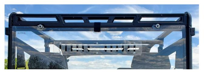
**Step 6:** After all clamps and hardware are attached, tighten the lock nuts on each bolt.
