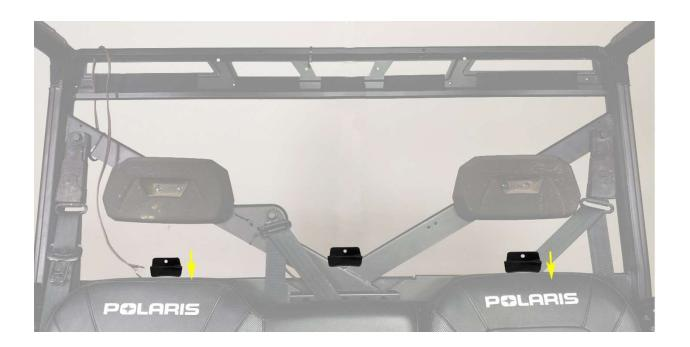
**Step 4:** As each clamp is placed into position, insert a hex head bolt thru a neoprene washer. Insert the bolt thru the back panel and thru the corresponding clamp. Insert a flat washer and lock nut onto the bolt. Only hand tighten at this time.
