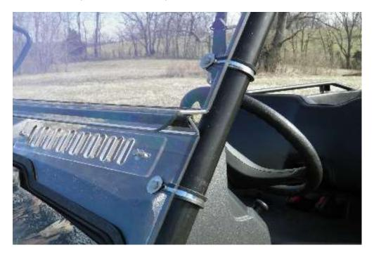
**Step 8:** When satisfied that the upper windshield section is positioned properly, tighten the knob bolts. Attach nuts to the knob bolts to hold in place.
