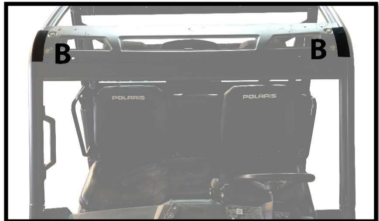
Figure 2: SHOWS PLACEMENT OF 6" VELCRO STRIPS (B)
