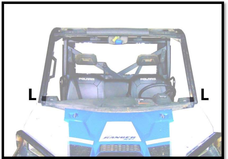
Figure 8: SHOWS PLACEMENT OF 3" VELCRO STRIPS. (L) FOR SMALL STRAP ON THE FRONT OF THE DOOR. PLACE TOWARD THE INTERIOR OF THE CAB NEXT TO DASH. IN WINDSHIELD TRACK.
