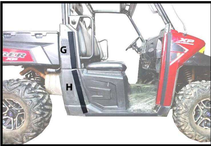
Figure 5: SHOWS PLACEMENT OF 14" AND 18" VELCRO STRIPS (G AND H)
