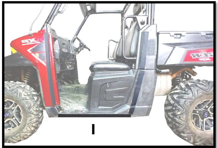
Figure 6: SHOWS PLACEMENT OF 29" VELCRO STRIP (I)
