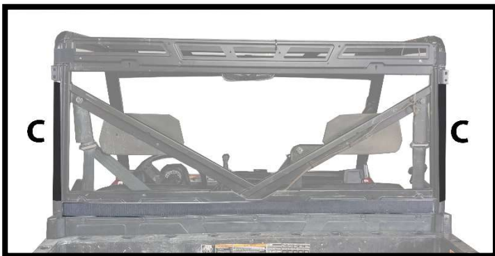
Figure 3: SHOWS PLACEMENT OF 18" VELCRO STRIPS (C)
