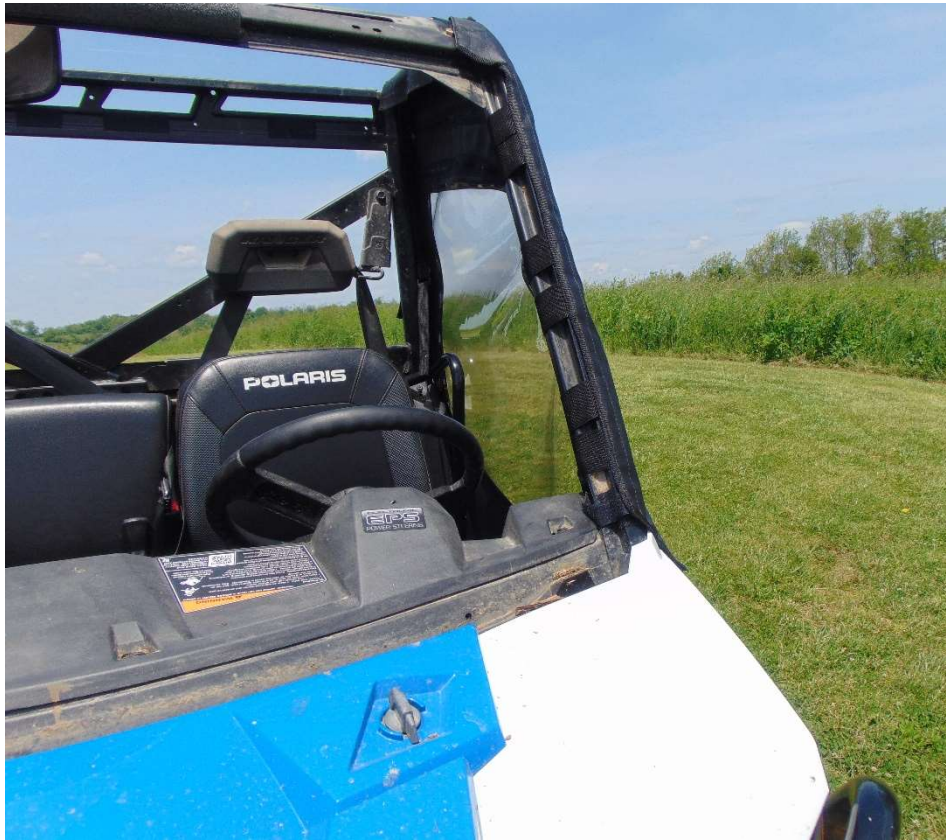
Figure 9: WHEN ATTACHING DOOR TO ADHESIVE VELCRO START WITH SIDE A. ALIGN BLACK TRIM ON THE DOOR PANEL TO THE EDGE OF THE INSET ROLL BAR. WRAP TABS AROUND THE INSIDE OF THE BAR AND ATTACH TO ADHESIVE VELCRO. CONTINUE TO ATTACH DOOR TABS AND STRAPS IN THE ORDER OF THE PICTURES AND VELCRO CHART.
