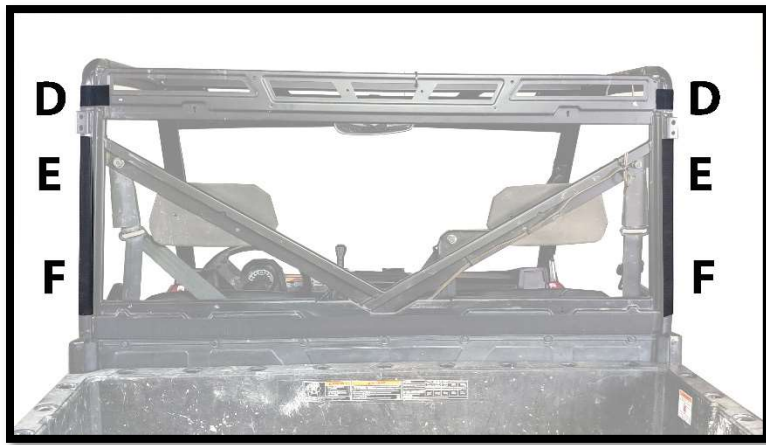
Figure 4: SHOWS VELCRO SEWN ON TO THE BACK PANEL FOR TABS D, E, AND F. WE INCLUDE THE VELCRO FOR THESE TABS ALSO, SO THAT YOU MAY REMOVE THE BACK PANEL AND USE ONLY THE DOORS
