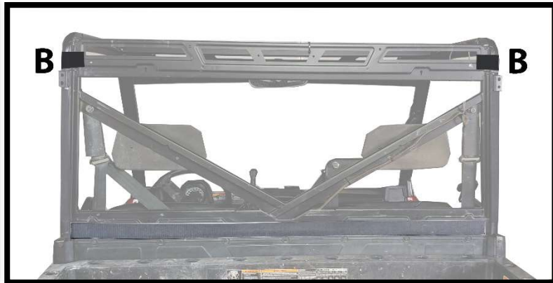
Figure 2: SHOWS PLACEMENT OF 6" VELCRO STRIPS (B).
