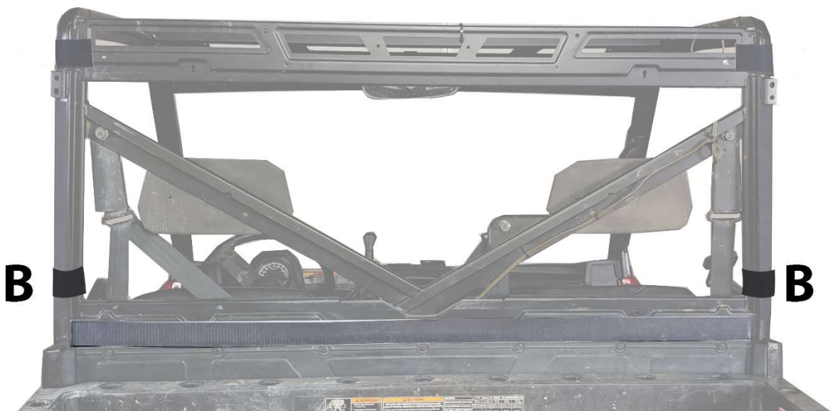
Figure 2: WRAP THESE VELCRO STRIPS AROUND THE ROLL BAR AND ATTACH DOUBLE-SIDED STRAPS.
