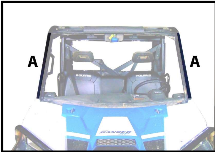
Figure 1: SHOWS PLACEMENT OF 26" VELCRO STRIPS (A) VELCRO STRAPS ON THE DOOR WILL WRAP AROUND ROLL-BAR AND CONNECT TO ADHESIVE VELCRO.
