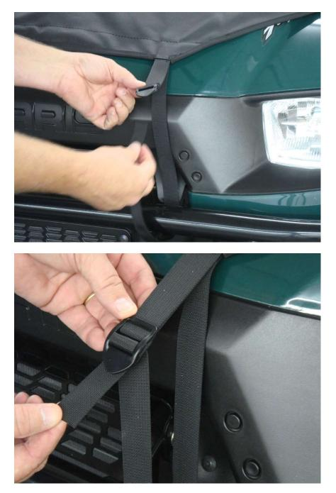
**Step 5:** Repeat all steps necessary to align and tighten the enclosure to the cab frame.
