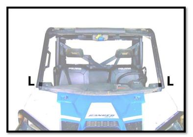
Figure 8: SHOWS PLACEMENT OF 3" VELCRO STRIPS. (L) FOR SMALL STRAP ON THE FRONT OF THE DOOR. PLACE TOWARD THE INTERIOR OF THE CAB NEXT TO DASH.
