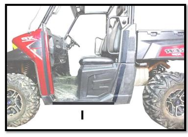
Figure 6: SHOWS PLACEMENT OF 29" VELCRO STRIP (I)
