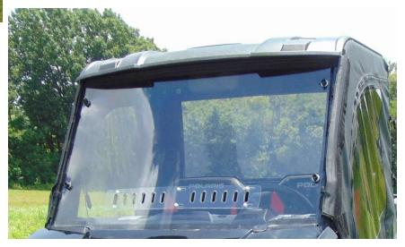
Figure 10: REINSTALL WINDSHIELD AND HARD TOP OVER THE DOOR KITS TABS AND STRAPS.
