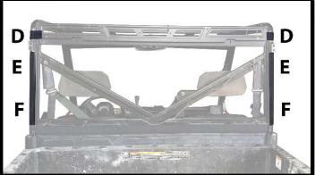
Figure 4: SHOWS PLACEMENT OF 4" AND 18" VELCRO STRIPS (D AND E) YOU CONNECT TABS E AND F TO THE 18" STRIP E.
