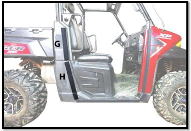
Figure 5: SHOWS PLACEMENT OF 14" AND 18" VELCRO STRIPS (G AND H)
