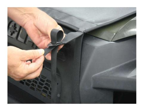
**Step 7:** Starting with the top Front Roll Bar Post Enclosure tabs pull outward and downward attaching tabs to the top 8" inch Velcro Strips as shown below. Repeat this process with the middle 8" and then lower 6" front roll bar enclosure tabs as shown making sure that the windshield is centered between the roll bar posts. Note: this step is best performed with an assistant attaching tabs on both sides of the windshield at the same time.
