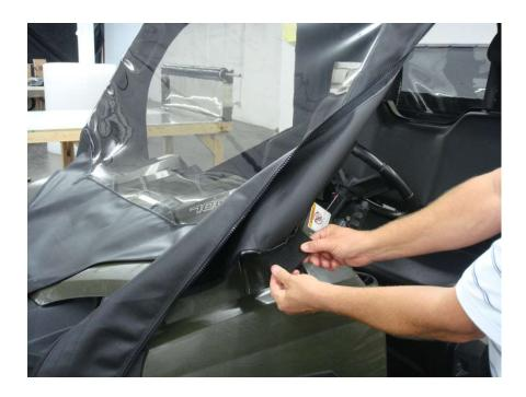
**Step 8:** Tighten Front Hood Straps by pulling downward from the buckle on both strap ends at the same time as shown below. This should tighten the Front Windshield and remove any major wrinkles.
