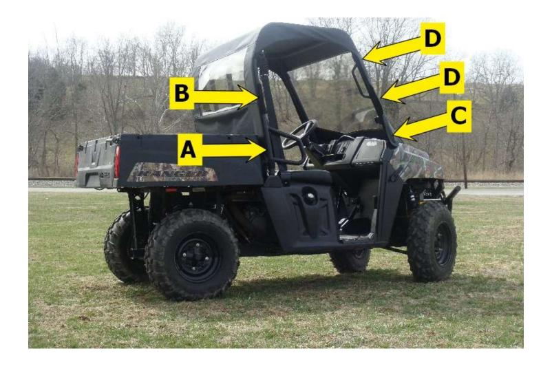
**Step 4:** After all adhesive hook strips have been attached, begin attaching the sewn in loop strips to the installed hook strips. Starting in the rear, align and square the enclosure to the cab frame as the hook and loop are joined.
