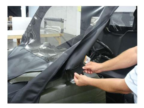
**Step 7:** Tighten Front Hood Straps by pulling downward from the buckle on both strap ends at the same time as shown below. This should tighten the Front Windshield and remove any major wrinkles.
