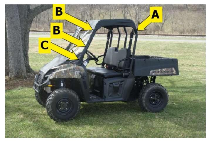
**Step 4:** After all adhesive hook strips have been attached, begin attaching the sewn in loop strips to the installed hook strips. Starting in the rear, wrap the double sided straps around the attached Velcro.
