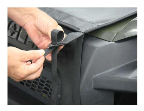
**Step 6:** Starting with the top Front Roll Bar Post Enclosure tabs pull outward and downward attaching tabs to the top 8" inch Velcro Strips as shown below. Repeat this process with the middle 8" and then lower 6" front roll bar enclosure tabs as shown making sure that the windshield is centered between the roll bar posts. Note: this step is best performed attaching tabs on both sides of the windshield at the same time, with the help of an assistant.
