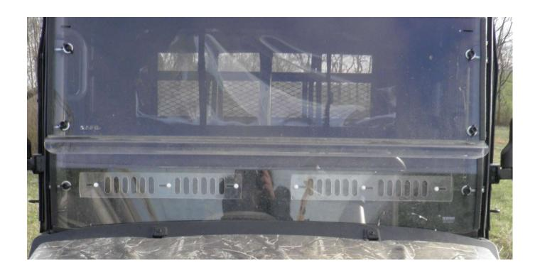
**Step 4:** When satisfied that the bottom windshield section is positioned properly, tighten the nuts on each clamp.
