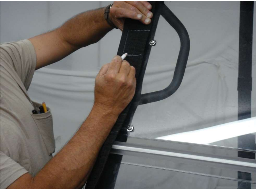
Figure 872 - Mark the Windshield Velcro Tabs for hard windshield Clamp locations
