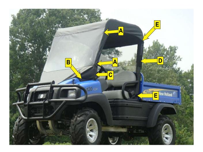
**Step 3:** After all adhesive Velcro strips are attached, place the enclosure on the cab frame and begin attaching the enclosure to the frame by first squaring the back of the enclosure to the rear of the cab frame and attaching the sewn-in Velcro loop behind the seats, the 8" tabs at each side of the back panel, and the straps at the bottom of the back panel.
