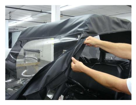
Attach tabs on either side of the windshield as shown above and below.
