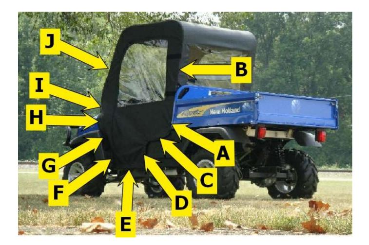
**Step 5:** After all adhesive Velcro strips are attached, begin attaching the enclosure by first squaring the back of the enclosure to the rear of the cab frame and attaching the sewn-in Velcro loop around the top of the back cross bar, the horizontal strip behind the seats, the 8" tabs at each side of the back panel, and the straps at the bottom of the back panel.
