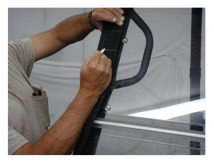
**Step 10:** Cut the webbing strip with household scissors. **AGAIN, DO NOT CUT INTO THE BINDING.** Seal the frayed edges with a lighter. Have a wet cloth handy to dab the edges.
