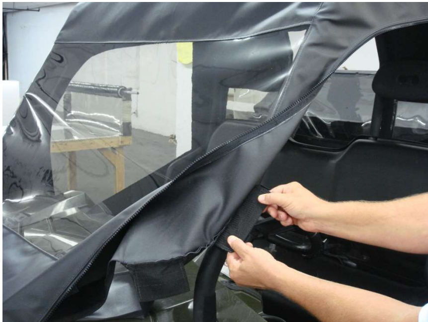
Attach tabs on either side of the windshield as shown above and below.
