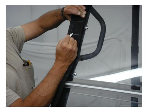
Step 3: Cut a section out around where your clamps will be positioned on the Velcro tab as shown. Be careful not to cut the binding.
