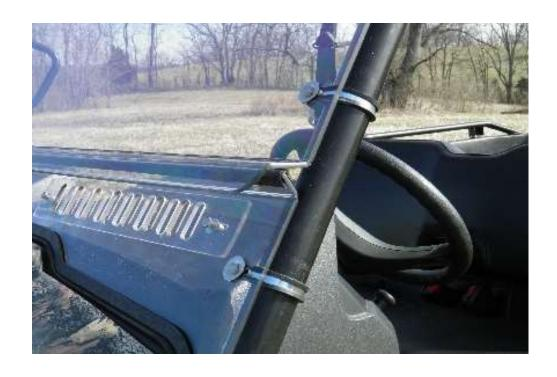
**Step 6:** Repeat Step 4 for each of the strap slots in the upper windshield section.
