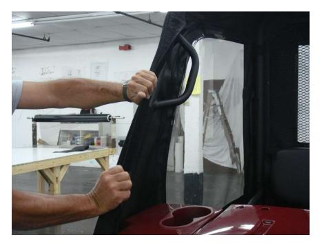
**Step 9:** The webbing/Velcro strip that runs the length of the front roll bars will need to be cut to accommodate the windshield clamps and the grab handle. With chalk, mark the webbing strip where cuts will be made. **DO NOT CUT INTO THE BINDING.**
