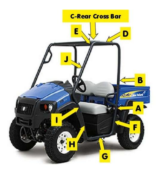
**Step 5:** After all adhesive Velcro strips are attached, begin attaching the enclosure by first squaring the back of the enclosure to the rear of the cab frame and attaching the sewn-in Velcro loop around the top of the back cross bar, the horizontal strip behind the seats, the 8" tabs at each side of the back panel, and the straps at the bottom of the back panel.
