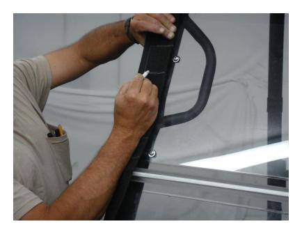
Mark windshield tabs where hard windshield clamps are located along the windshield Roll Bar
