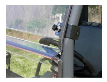
**Step 4:** When satisfied that the bottom windshield section is positioned properly, tighten the two clamps' nuts on each clamp.
