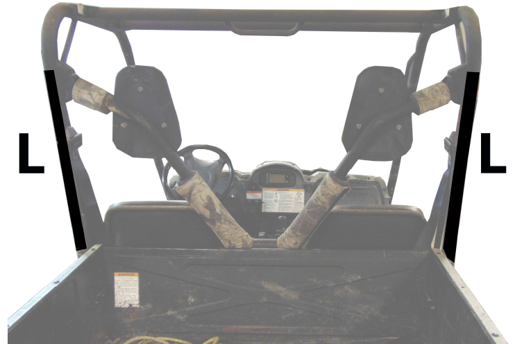
Figure 4: Shows placement of Velcro strips down the back of the roll bar. If you have a back panel the Velcro for this tab is sewn down the back of the back panel.
