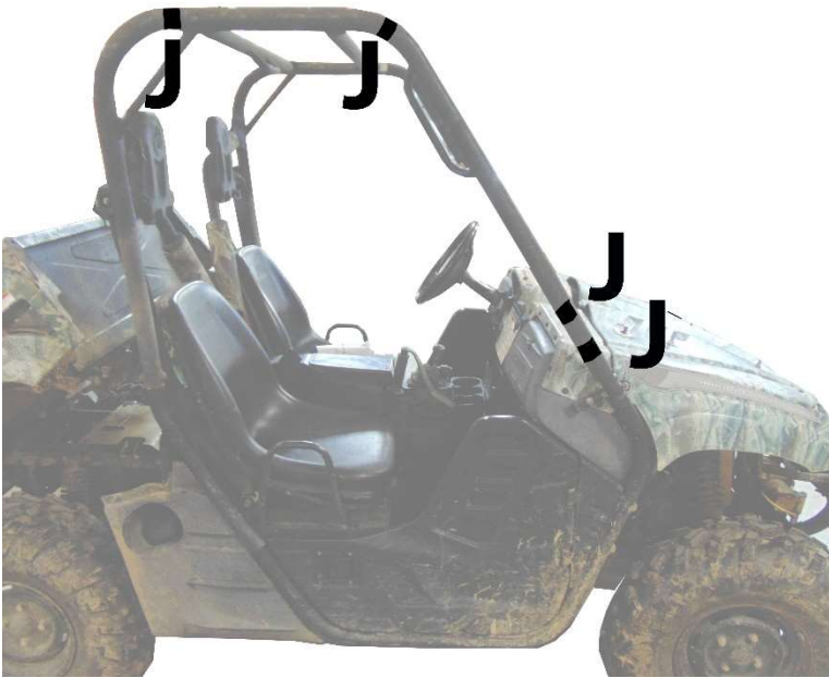
Figure 5: Adhesive strips J will wrap around the bar, The double sided tab on the window of the door kit is for the side grab bar, some UTV may not have this side grab bar.
