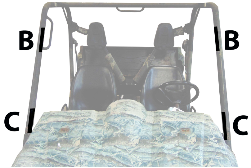
Figure 2: Place these strips more towards the inside of the roll bar. Tabs on the front of the door kit will wrap around the roll bar.
