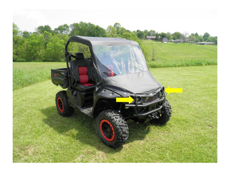
**Step 3:** Straps on front of windshield/top wrap around front bumper and back thru buckle.
