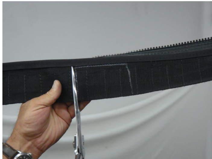
Figure 7.3 – Cut a 2" section out around where your clamps will be positioned on the Velcro Tab – be careful not to cut the binding
