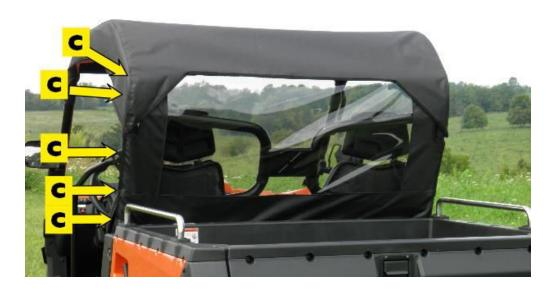
**Step 3:** After all adhesive hook strips are attached, begin attaching the enclosure to the cab frame. As you attach the hook and loop, square each panel to the frame.
