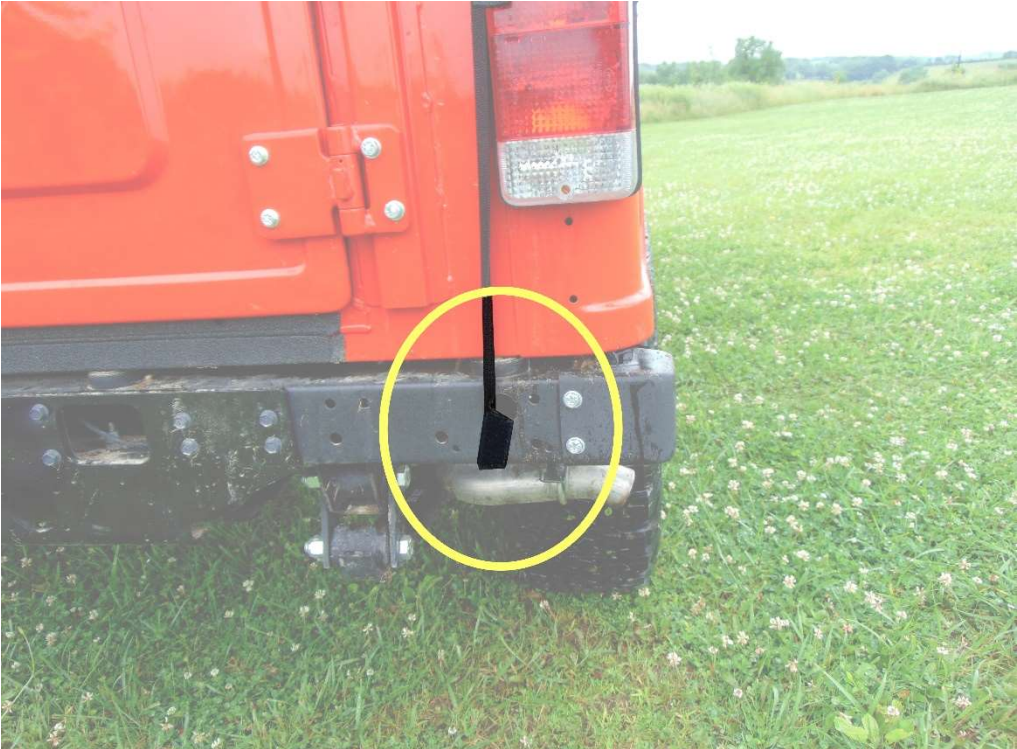
Figure 1: WRAP THE DOUBLE SIDED STRAPS THROUGH THE LARGE ROUND HOLE IN THE BUMPER.
