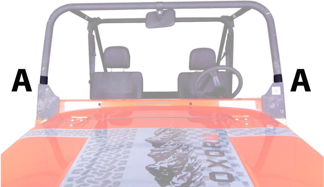
Figure 2: WRAP THESE VELCRO STRIPS AROUND THE ROLL BAR AND ATTACH DOUBLE-SIDED STRAP.
