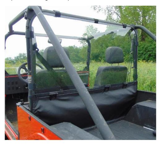
**Step 7:** Feed the tabs on the fabric lower panel from the inside of the vehicle through the slots cut on the bottom of the back panel. Secure the tabs on the sewn in loop.
