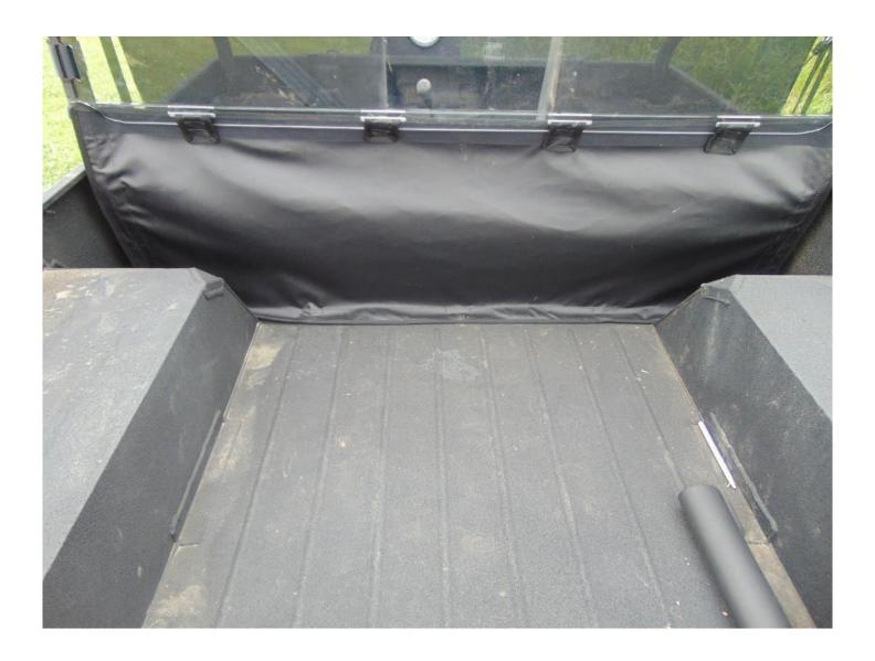
**Step 8:** Apply the two 20" adhesive velcro strips down the roll bars corresponding to the sewn in loop on the sides of the fabric lower panel.
