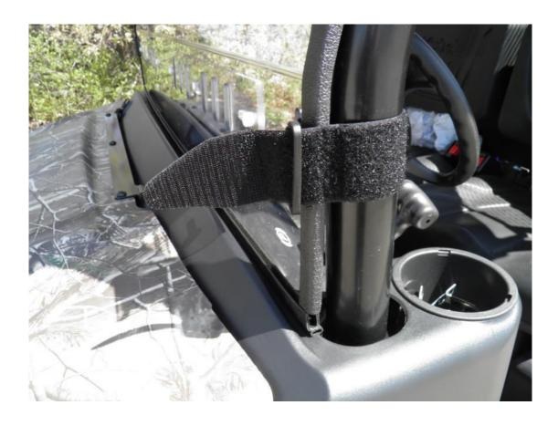
**Step 6:** Adjust the straps as needed to align the back panel.
