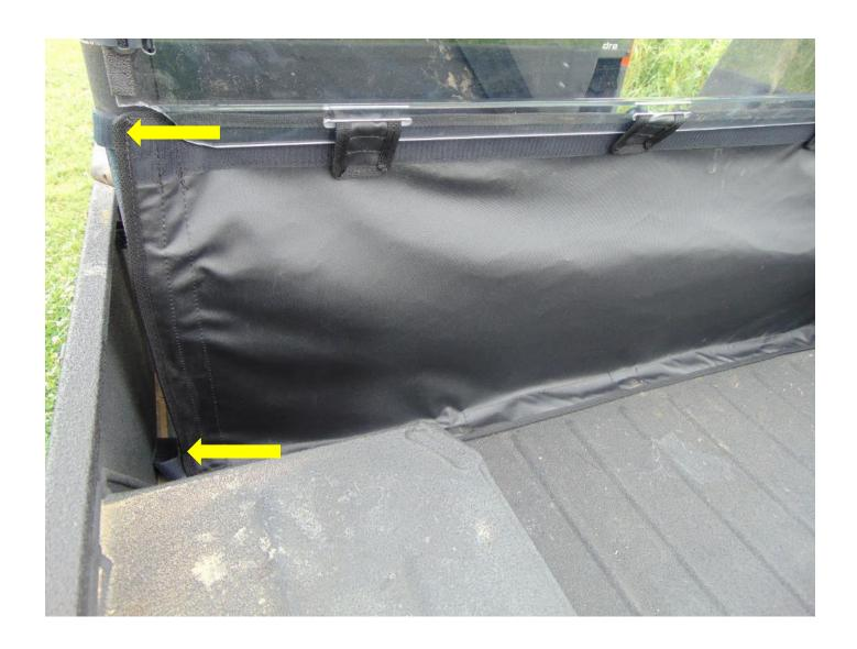
**Step 9:** Wrap the double-sided straps around the adhesive velcro to secure the top sides of the fabric lower panel.
