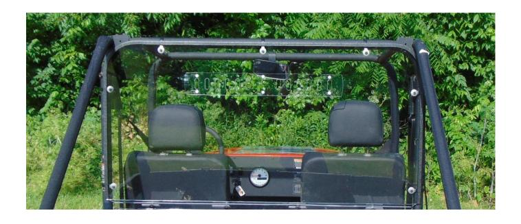
**Step 3:** Prepare hardware for each of the loop clamps. Insert a neoprene washer onto the hex head bolts. When installed, the bolts with neoprene washer will go thru the pre-routed holes in the windshield and into the clamps. The clamps will be tightened with a flat washer and lock nut.
