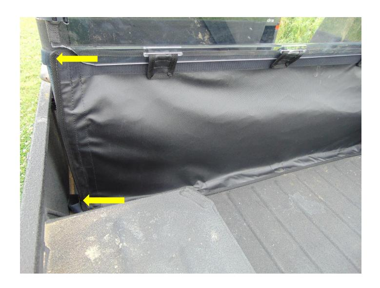
**Step 10:** Wrap the double-sided straps around the adhesive velcro to secure the top sides of the fabric lower panel.
