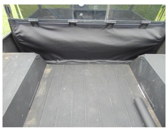
**Step 9:** Apply the two 20" adhesive velcro strips down the roll bars corresponding to the sewn in loop on the sides of the fabric lower panel.
