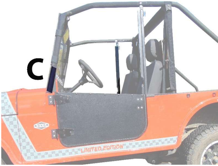
Figure 3: Shows placement of 8" Velcro strips C.
