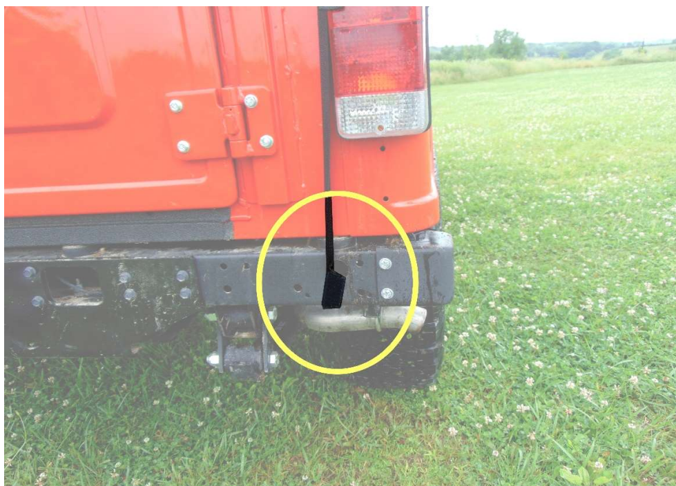
Figure 2: WRAP THE DOUBLE SIDED STRAPS THROUGH THE LARGE ROUND HOLE IN THE BUMPER
