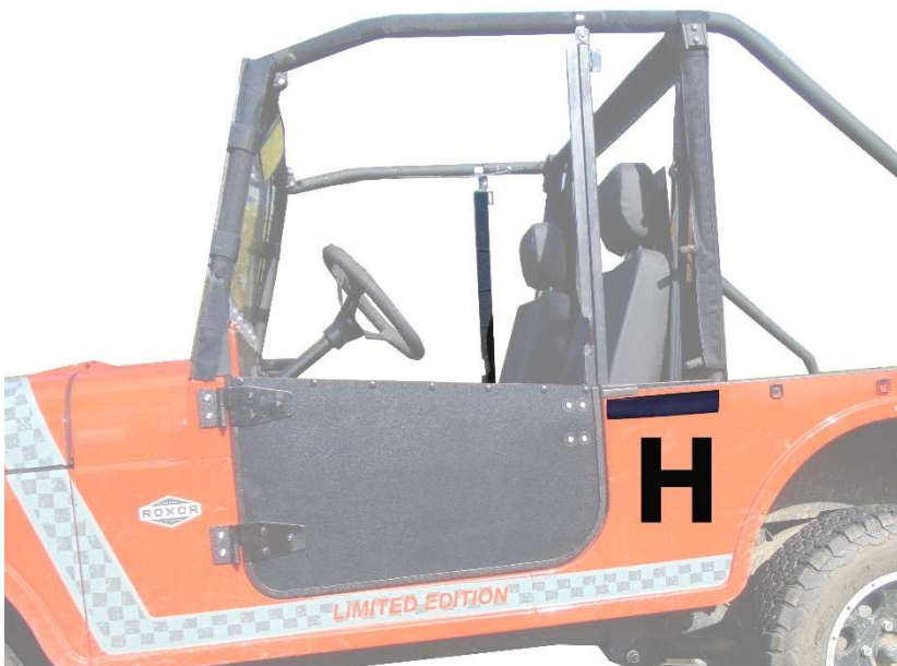
Figure 7: Shows position of 11" Velcro strips H.
