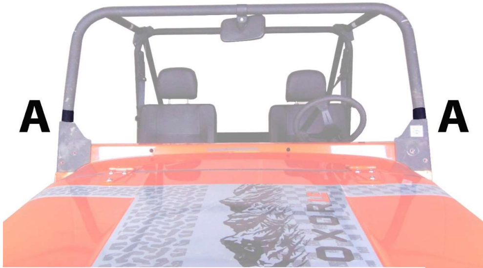
Figure 1: WRAP THESE VELCRO STRIPS AROUND THE ROLL BAR AND ATTACH DOUBLE-SIDED STRAP.
