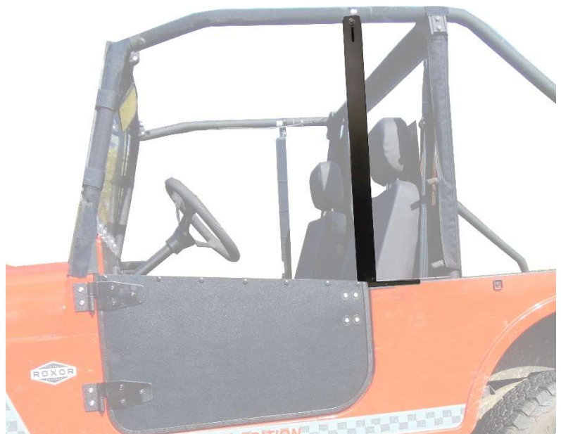
STEP TWO: Set side bar on the UTV with the lower fork to the inside of the cab. Between the UTV body and the seat bar.
