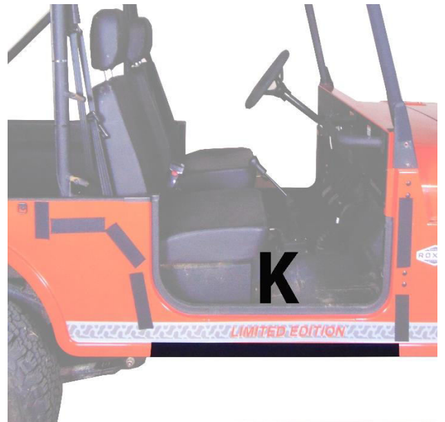
Figure 6: Shows position of Velcro strips K.
