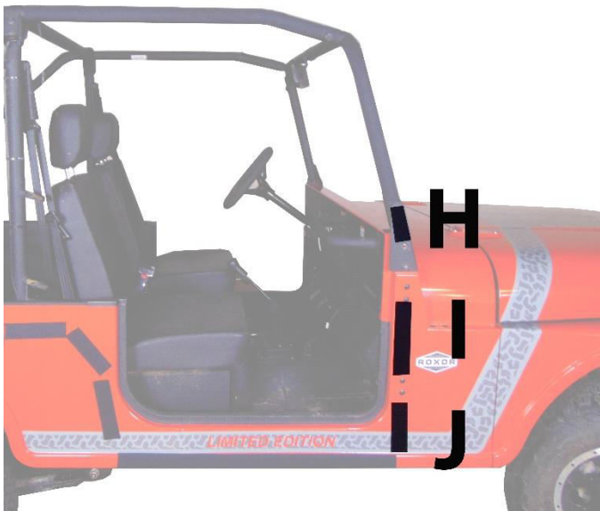
Figure 5: Photo shows placement of Velcro strips H I and G.
