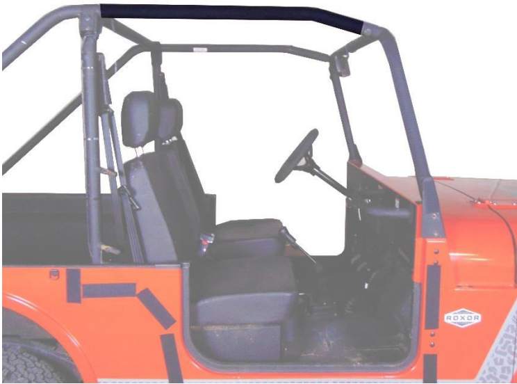
Figure 1: Shows placement of 36" Velcro strips A.
