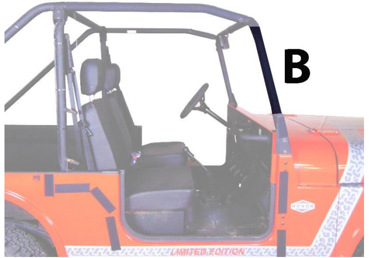
Figure 2: Shows placement of 21" Velcro strips B.
