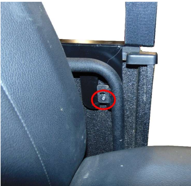
STEP ONE: Remove factory bolt from seat handle bar.
