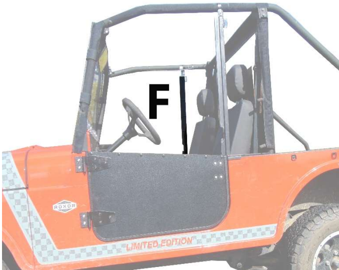
Figure 5: Photo shows placement of Velcro strips F.
