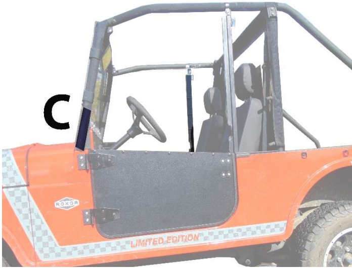
Figure 3: Shows placement of 8" Velcro strips C.
