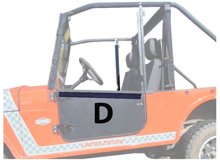
Figure 4: Shows placement of 32" Velcro strips D.
