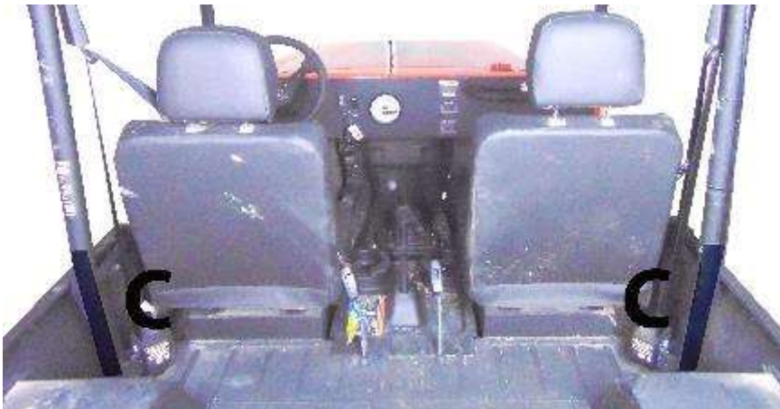
Figure 3: Shows position of 17" Velcro strip C. The bottom back of the back panel will attach to this Velcro strip.
