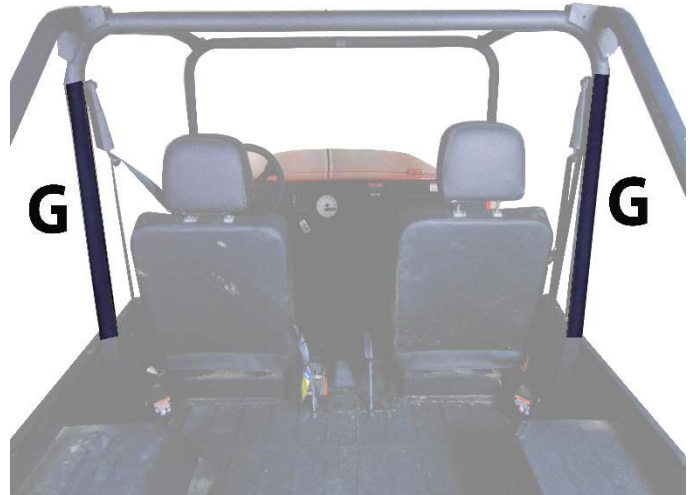
Figure 6: Shows position of Velcro strips G.
