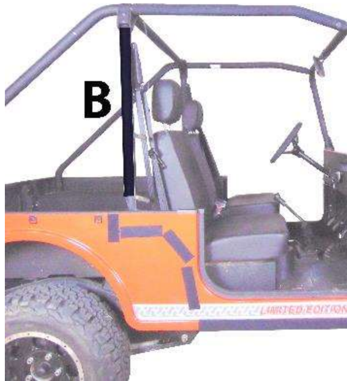
Figure 2: Shows position of 32" Velcro strips B. Wrap the edge of the back panel around the side of the roll bar. The drivers side will get the same strip in the same position.
