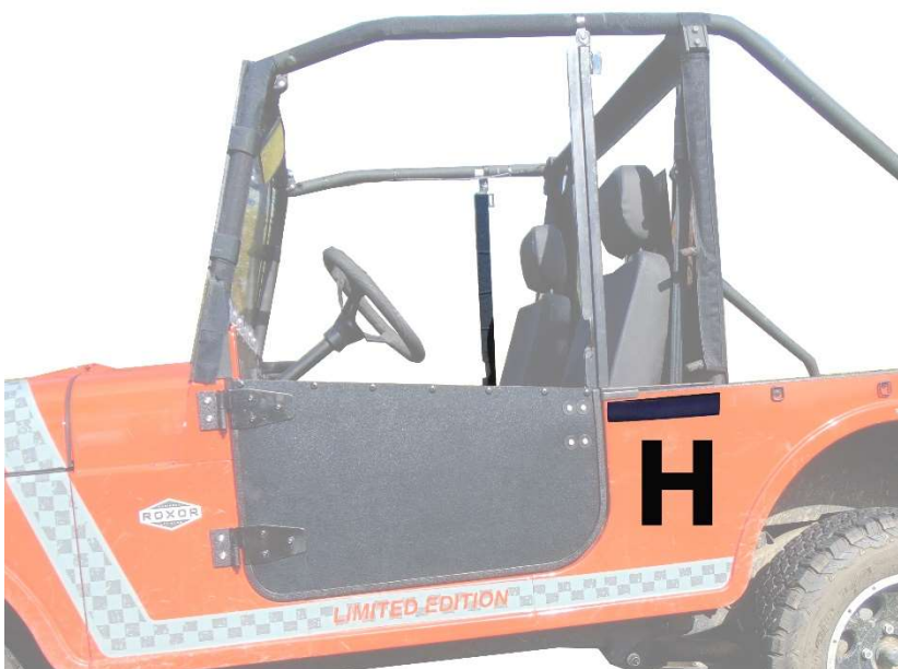
Figure 7: Shows position of 11" Velcro strips H.
