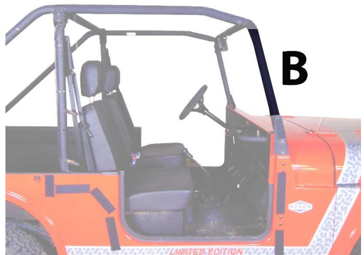
Figure 2: Shows placement of 21" Velcro strips B.
