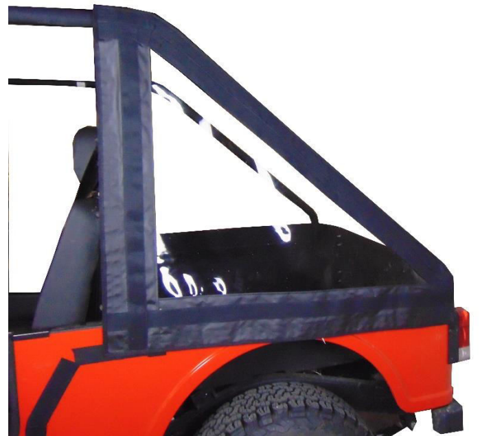
Figure 4: The triangle panel should line up with the slant of the back roll bar.
