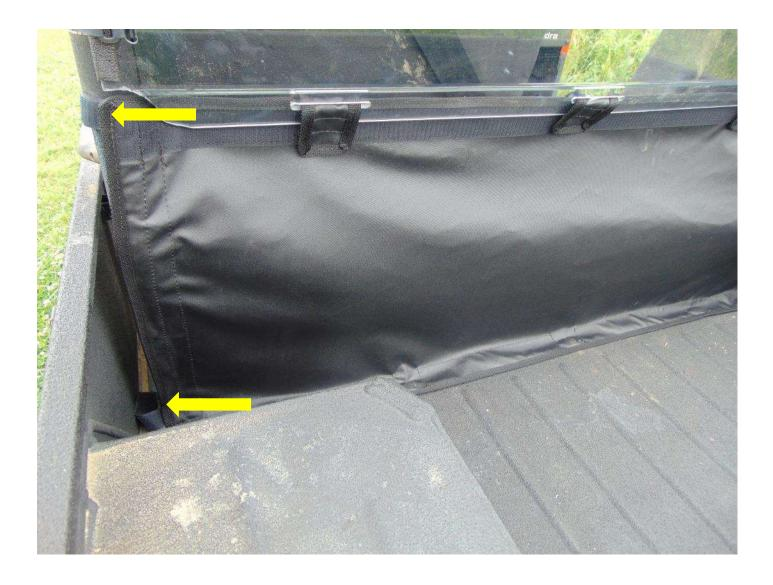
Step 9: Wrap the double-sided straps around the adhesive velcro to secure the top sides of the fabric lower panel.Step 10: Remove the protective plastic paper from each side of your windshield.
