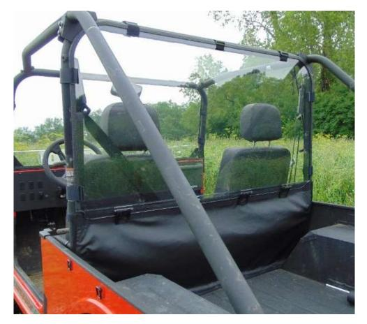
**Step 7:** Feed the tabs on the fabric lower panel from the inside of the vehicle through the slots cut on the bottom of the back panel. Secure the tabs on the sewn in loop.
