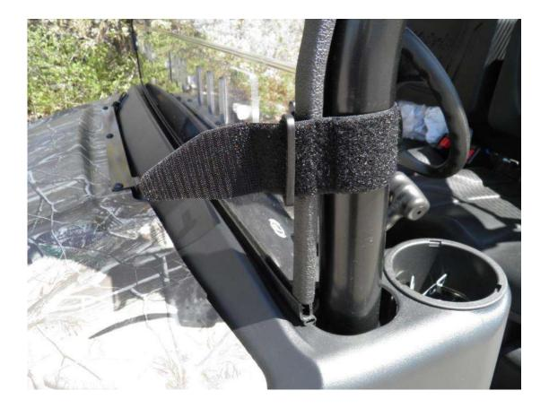
**Step 6:** Adjust the straps as needed to align the back panel.
