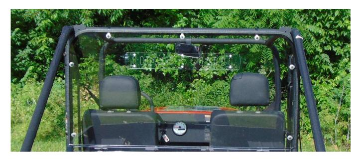
**Step 3:** Prepare hardware for each of the loop clamps. Insert a neoprene washer onto the hex head bolts. When installed, the bolts with neoprene washer will go thru the pre-routed holes in the windshield and into the clamps. The clamps will be tightened with a flat washer and lock nut.
