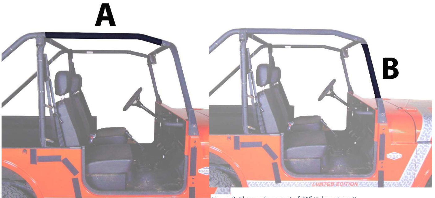
Figure 1: Shows placement of 36" Velcro strips A.
