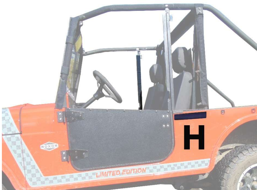
Figure 7: Shows position of 11" Velcro strips H.
