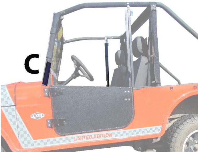
Figure 3: Shows placement of 8" Velcro strips C.
