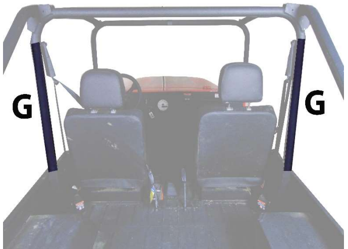
Figure 6: Shows position of Velcro strips G.
