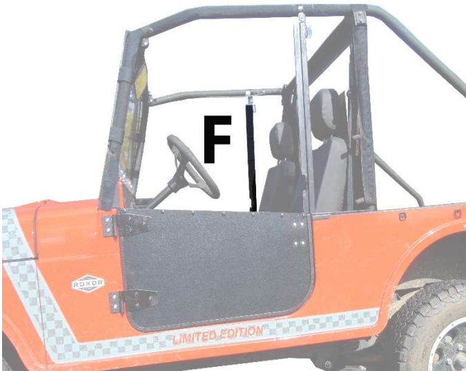
Figure 5: Photo shows placement of Velcro strips F.
