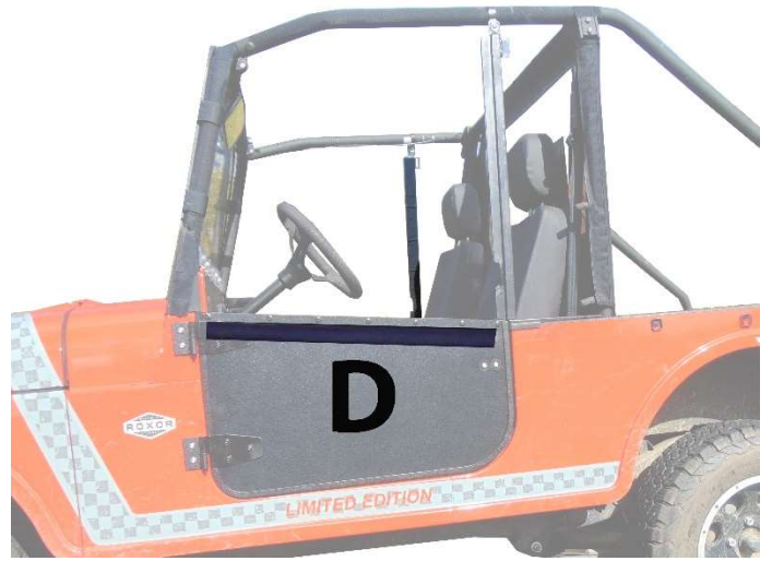
Figure 4: Shows placement of 32" Velcro strips D.
