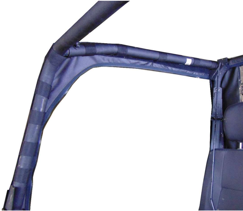
Figure 7: Sewn on Velcro strips on the top and front of the door should be lined up first with the door kits binding resting on the edge of the roll bar. Once the door kit is lined up properly you may then wrap the straps around the bar and attach to adhesive Velcro.
