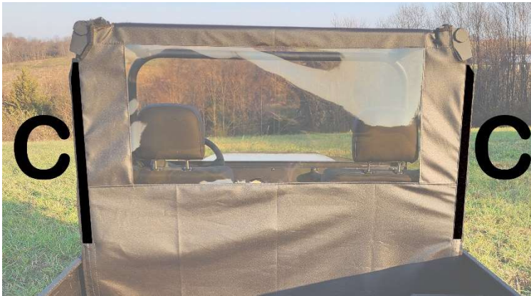
Figure 3: Shows placement of 29" Velcro strips C. The tabs on the back of your doors will wrap around the roll bar and attach to the Velcro strip.
