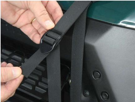
**Step 5:** With the enclosure properly aligned to the cab frame, tighten the front straps by pulling downward from the buckle on both strap ends at the same time as shown.
