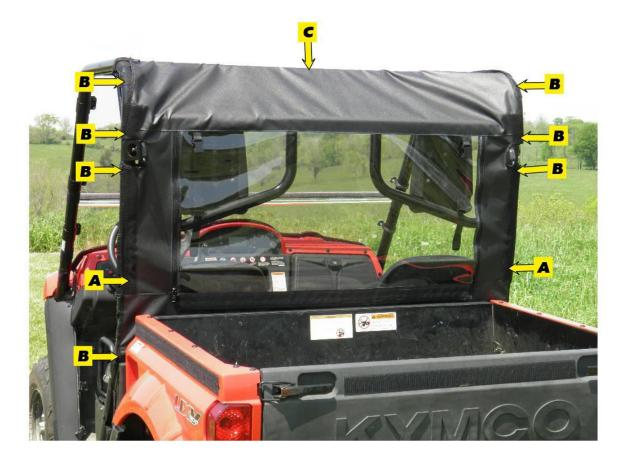
**Step 3:** After all adhesive hook strips are attached, begin attaching the enclosure to the cab frame. As you attach the hook and loop, square each panel to the frame. <u>PLEASE NOTE, FOR MAXIMUM ADHESION, ALLOW THE ADHESIVE</u> <u>HOOK TO ADHERE TO THE FRAME FOR 24 HOURS BEFORE PULLING AGAINST THE HOOK WITH THE LOOP STRIPS.</u>
