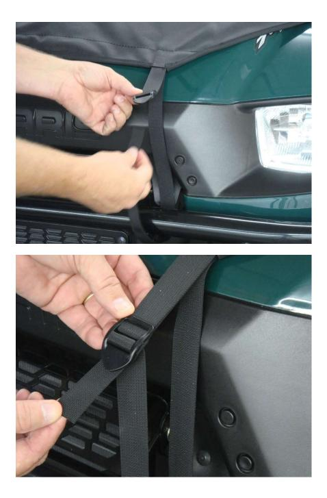
**Step 5:** With the enclosure properly aligned to the cab frame, tighten the front straps by pulling downward from the buckle on both strap ends at the same time as shown.
