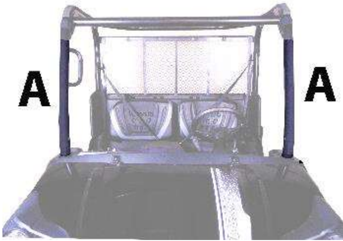
Figure 1: Shows placement of Velcro strips A. Attach soft Velcro on the top of the door, pull the door around so that the seam lines up to the middle of the roll bar.
