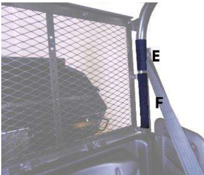
Figure 5: Photo shows placement of 5" and 15" Velcro strips E and F. You will position identical strips on the passenger side.
