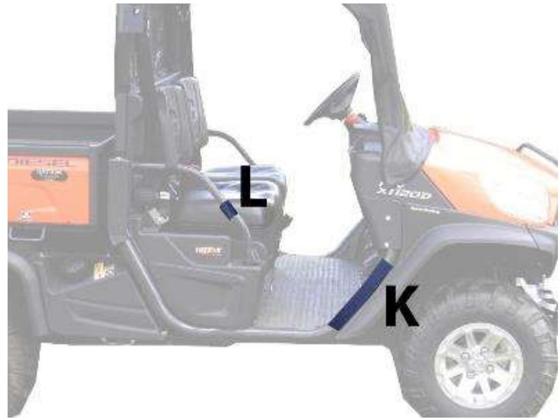
Figure 8: Shows position of 15" and 3" Velcro strips K and L, you will place identical strips on the drivers side.
