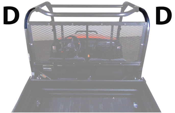
Figure 4: Shows placement of Velcro strips D.
