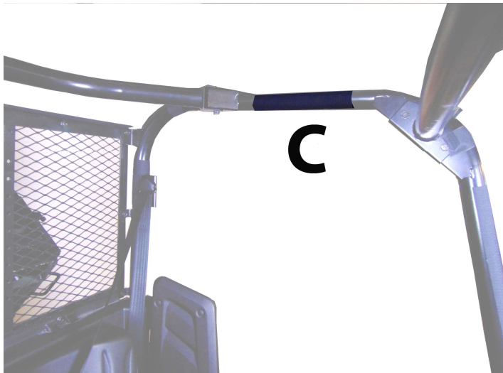
Figure 3: Shows placement of Velcro strip C
