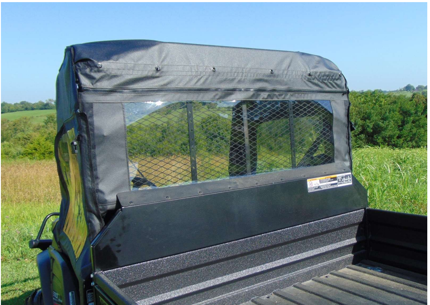
Notice how the back panel is smooth and tight across the back of the UTV, the screws fit perfectly in the grommets. If installed correctly your back panel should resemble the photo.
