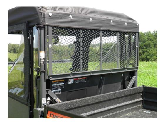
**Step 4:** Before mounting, pull the protective paper from the edge of each side of the rear panel. If the rear screen will be re-mounted, pull the protective paper from that side of the rear panel.
