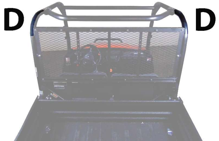
Figure 4: Shows placement of Velcro strips D.
